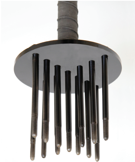
Figure 1. The head of the spiked shear vane. The blades of a conventional shear vane are replaced by rows of tapered steel spikes.
