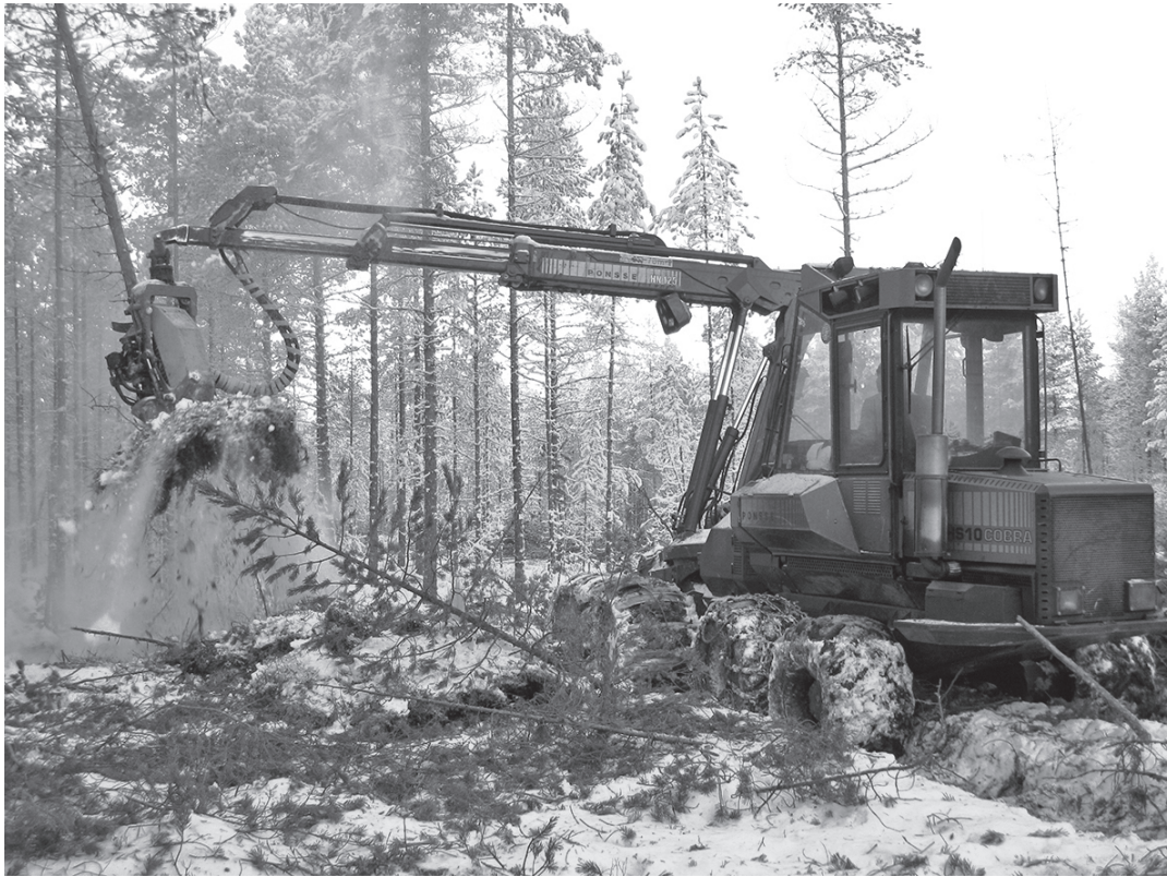
Fig. 12. Complete tree cutting with a Ponsse Cobra single-grip harvester in the experimental stand of this study (Photo: Juha Laitila).
