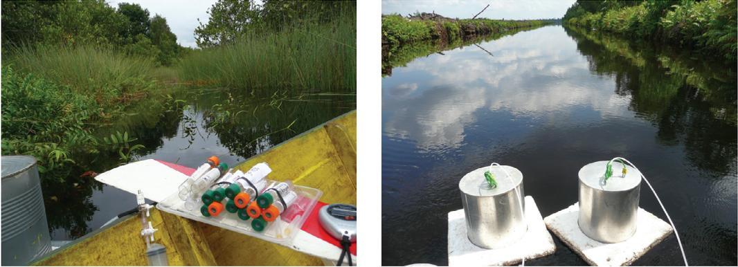
Figure 1. Typical view inside settled canals at the Kalimantan (left) and Kampar (right) sites with some gas flux monitoring equipment in use.
