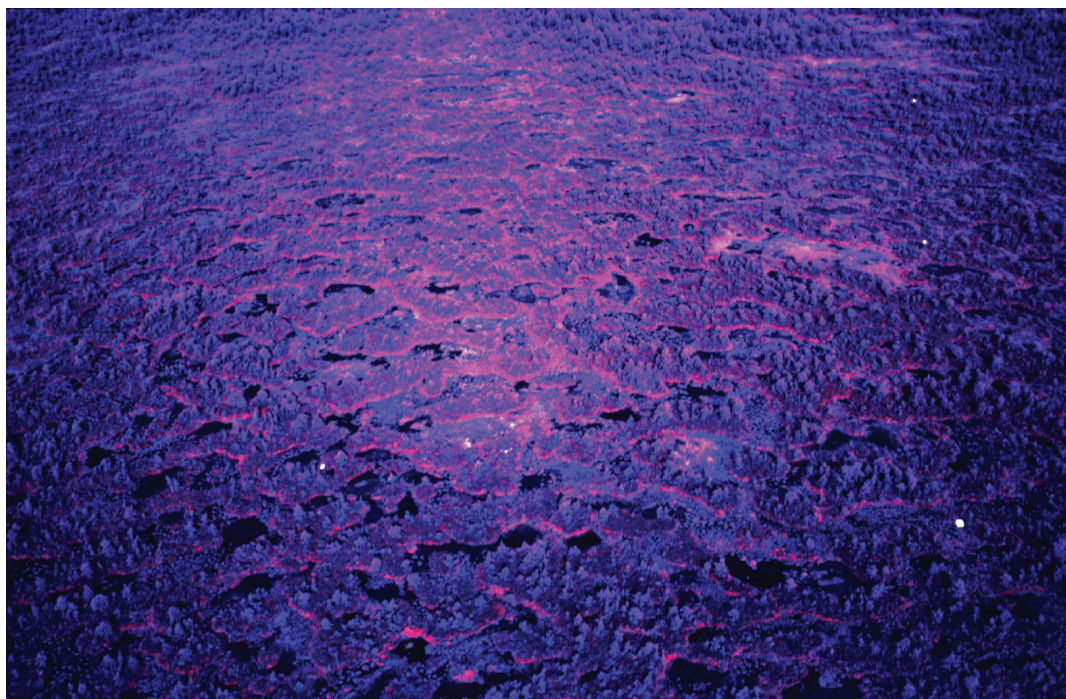
Fig. 12. Color-infrared picture over Teosaare Bog showing an enhanced hot-spot effect at scene center. Compare with Fig. 6.
