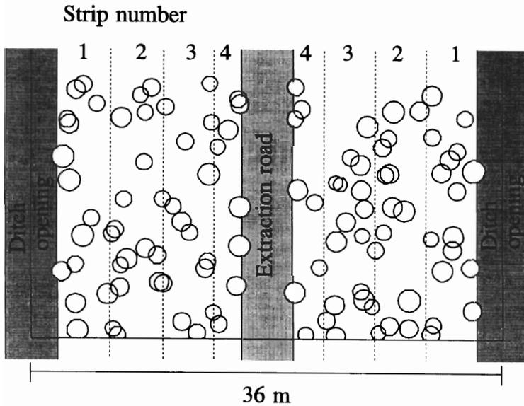
Fig. 1. The model stand was a 36 m wide rectangular plot between two adjacent ditches. The ditch lines were 4 m wide. A 4 m wide extraction road was cut in the first thinning. The remaining basal area was defined separately for 4-m strips parallel to the ditches.
