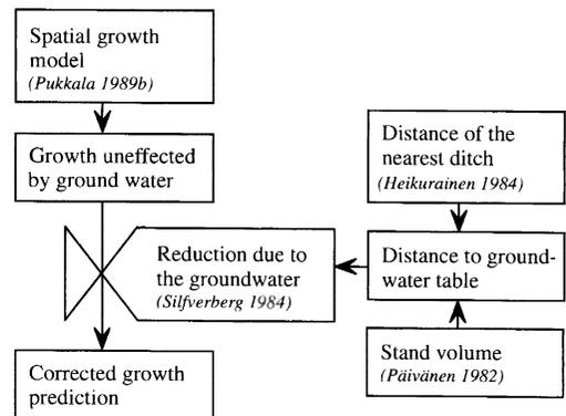
Fig. 2. Steps in the calculation of growth prediction with the model of Miina et al. (1991). The mentioned studies have been used in the formulation of the sub-models.
